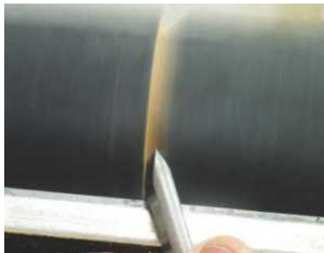
▲ Pic.8 The tool is presented with the left-hand bevel at right angles to the work and the longer point down. Lift the handle to slice into the wood
